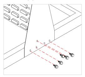
**4.** Hang the panels (5) in the holders (4) provided and tighten the screws (10) to secure them.
