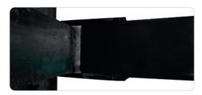
4. Verify that the fork extensions are firmly secured on the forks.
