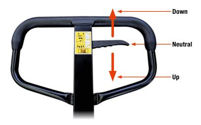
To raise the fork, set the lever in the "UP" position (lever down).
