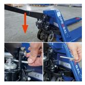
5. Move the drawbar down to release the tension. Now remove the safety bolt.
