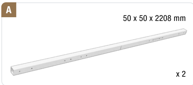
Lateral roof beam
