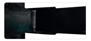
4. Verify that the fork extensions are firmly secured on the forks.
