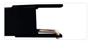
3. Put the locking bolts behind the back of the forks through the hole provided and secure them.
