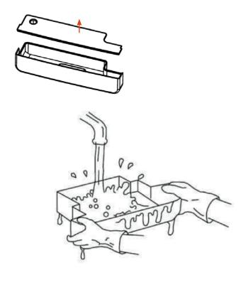
To ensure the longevity and reliability of this dryer, check the condition of the filters regularly (at least every two months) and clean them with a light jet of compressed air if necessary. To clean the filters, remove the water collection container and slide the cover upwards. Be careful not to touch the paper on the filter and clean the filter carefully as it is very delicate. Never expose filters to moisture and make sure they always stay dry.
