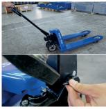
7. Now test the function: Pump the handpiece a few times so that the fork lifts. Move the lever up so that the fork lowers again.
