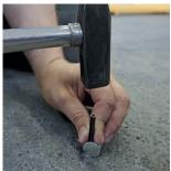
2. Use a hammer to drive in the locking pin on one side and insert the axle bolt into the holder. Make sure that the hole in the axle bolt is facing forward. If the hole is on the other side, insert the axle bolt from the other side.
