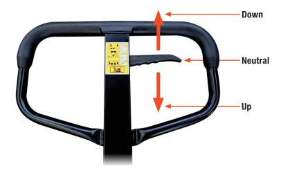
To raise the fork, set the lever in the "UP" position (lever down).
