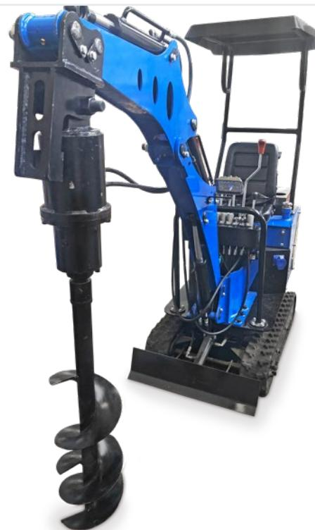
4. Connect the two hydraulic hoses to the free hydraulic connections on the excavator.
