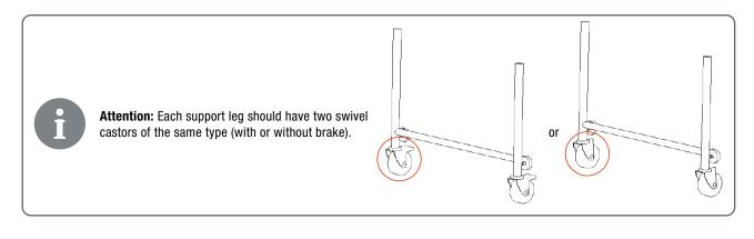
3. Take the roller track out of the box and attach the feet.
